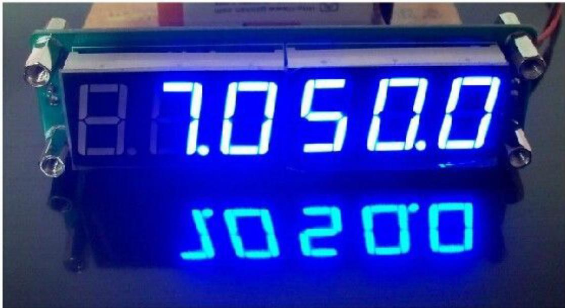
PLJ - 6 leds - A is designed for the HAM friends of cost-effective six LED display module, frequency is mainly used for transceiver equipment such as frequency values show, also can be used in the conventional frequency measurement.
