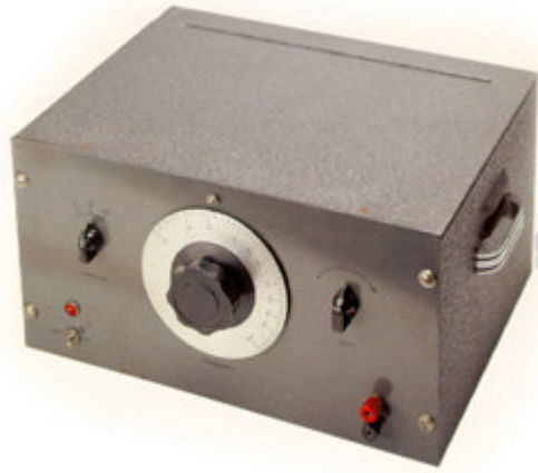
Bill Hewlett 200A Oscillator Prototype as shown in the MEASURE "Wrapping it up" issue Courtesy of Hewlett Packard Company
