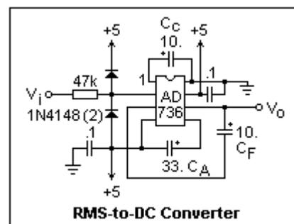
smooth the output. The values of the capacitors determine the averaging times and bandwidths, as is obvious. The values shown here are good for general service.  $C_A$  can range up to  $150\mu\text{F}$ , and  $C_F$  up to  $100\mu\text{F}$ , if desired. The **AD736** will handle crest factors up to 5.
