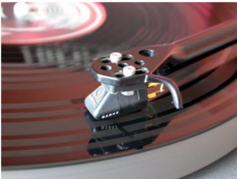
Once you've aligned your cartridge with one of the protractors you are ready to run through the tests. If you are unfamiliar with test records the first thing you will notice are the widely spaced locked grooves; each 'band' contains a different test and you have to cue them individually.
